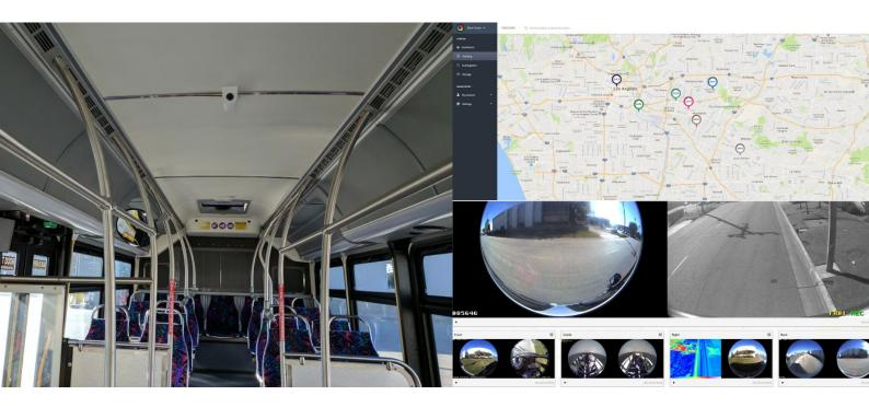
and noise level, temperature, GPS position, GPS directions and GPS velocity. The sensor readings are essential to trigger automated alerts to the control room for example if a bus is involved in an accident or has deviated off course.
